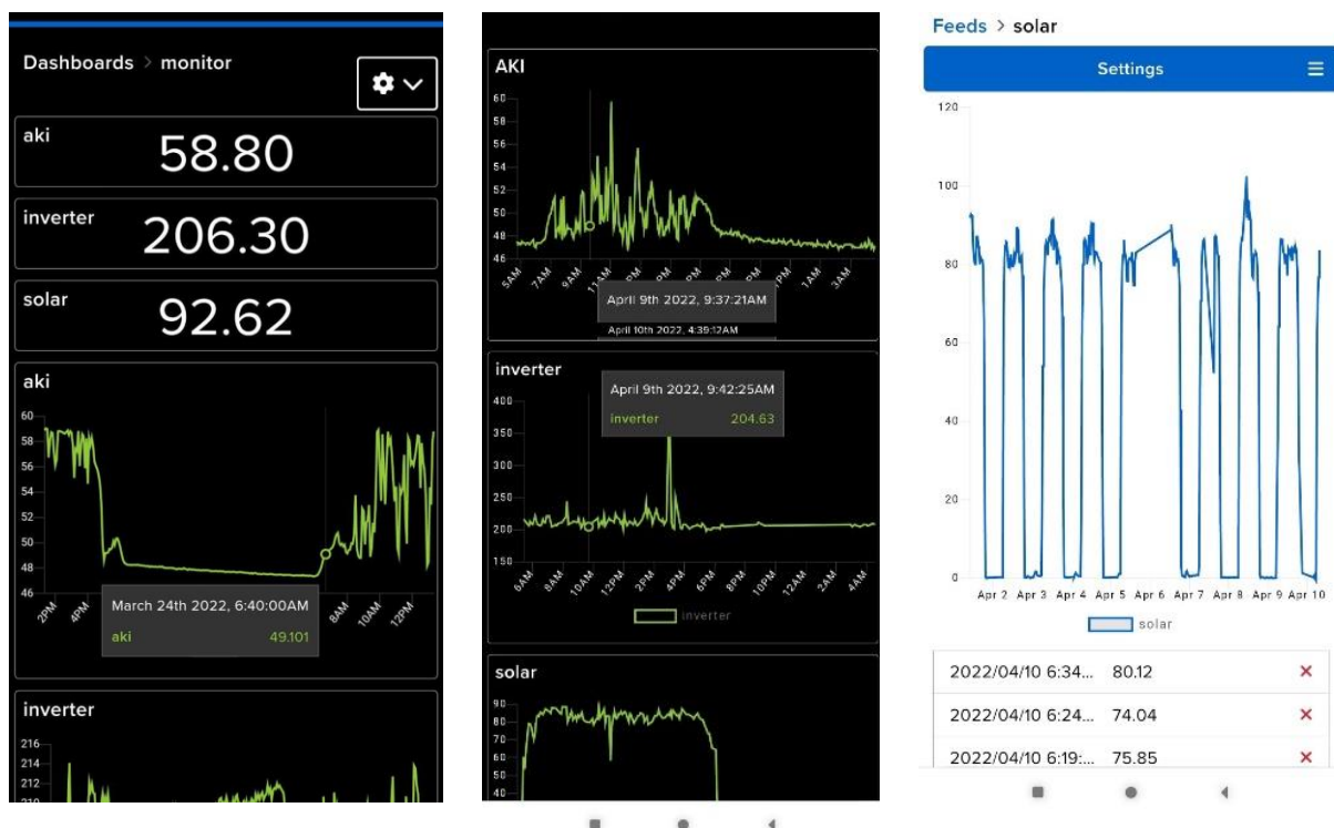
Figure 6. IoT Monitoring Interface
