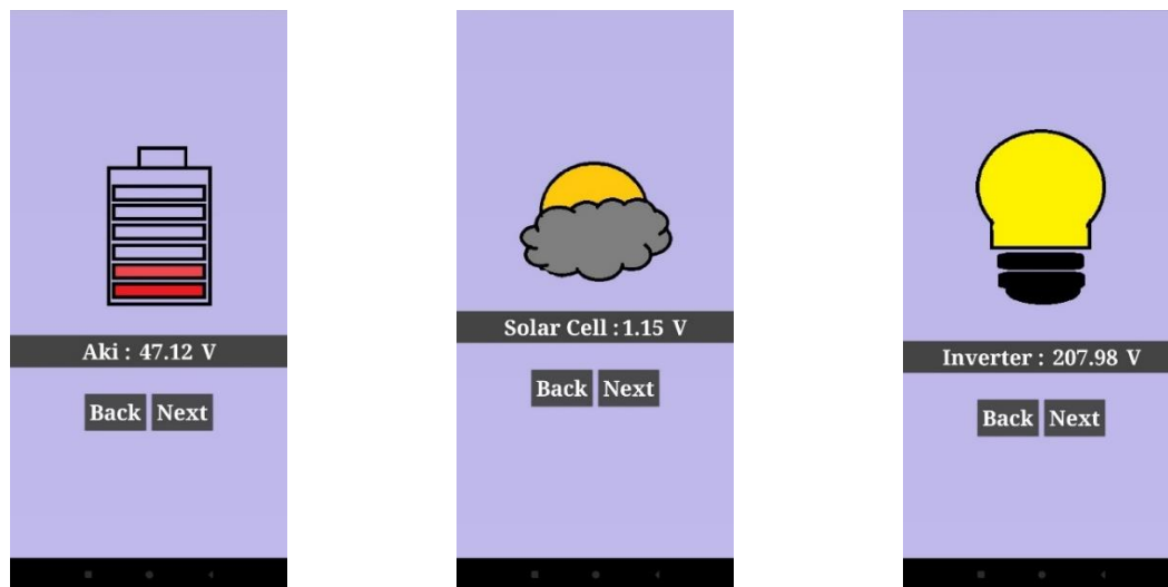
Figure 3. IoT monitoring of PV system installed in RSI Siti Khadijah Palembang
